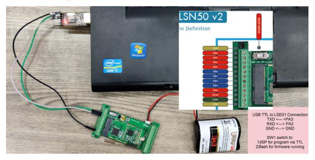
In the PC, you need to set the serial baud rate to **9600** to access the serial console for LSN50. LSN50 will output system info once power on as below:
