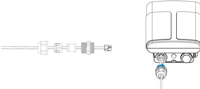
For DC or solar power supply, remove the protective cap of the power connector and rotate the DC power cable into the power connector.
