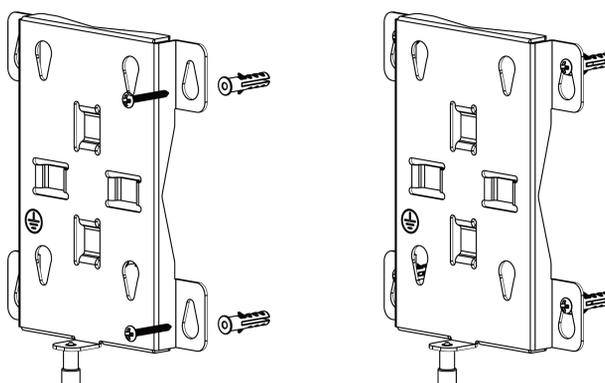
E. Hang the device to the mounting bracket via bracket mounting screws on the back of the device, then screw the bracket screw to the bottom of the device.
