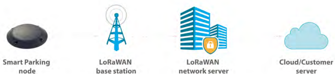
Figure : Simplified Smart Parking network architecture
