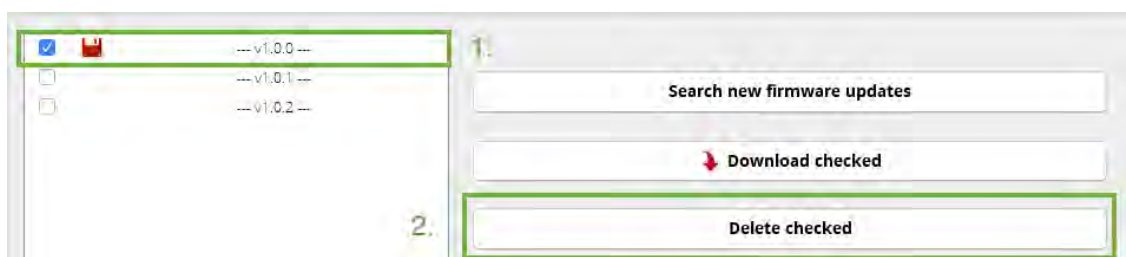
Figure : Firmware deletion process for Smart Parking v2
