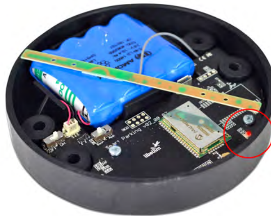
Figure : The red LED blinks once to indicate ready-to-install state
