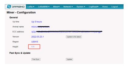
This may be related to the current block height, if the device is synchronizing to the latest height or if the device block height is much lower than the current height as the above picture like '1 1', the QR code generation may fail
