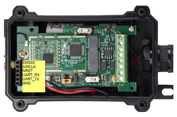
In the PC, you need to set the serial baud rate to **9600** to access the serial console for LSE01. LSE01 will output system info once power on as below:
