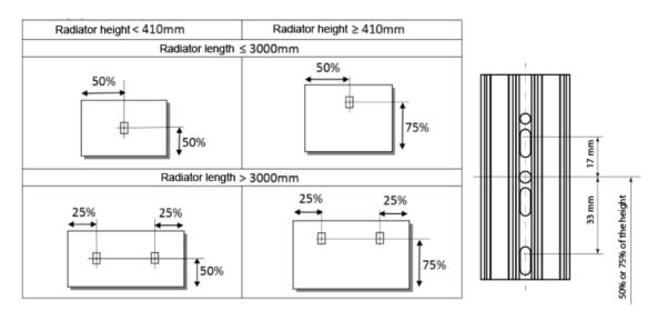
Wall mounting, the remote sensor is mounted on the radiator and the heat cost allocator is mounted on the wall.
