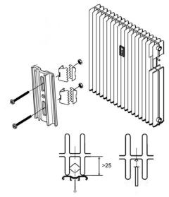
• For a better fixing use 2 x 2 spreadable brackets, fix the aluminium profile by passing the screws through the oblong holes and shorten them if necessary.
