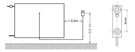
Wall mounting must be carried out if the design of the radiator does not allow sufficient contact with the conductive elements or if the radiator is smaller than 250 mm in height or if for reasons of aesthetics or water splashes, the heat cost allocator cannot be mounted on the radiator.
