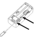
Return the heat cost allocator and plug the connector of the remote sensor into the interface inside the heat cost allocator. Insert the remote sensor cable into the groove provided up to the slot of housing.
