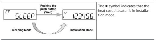
Once installed on the back plate or the wall, the heat cost allocator switches automatically into operating mode at the second transition of midnight.
