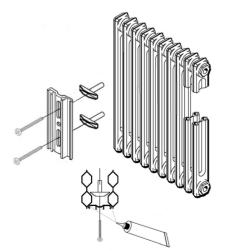
In the case of cast iron radiators, the contact surfaces of the aluminium mounting plate should be coated with heat-conducting paste before fixing.
