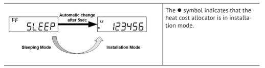
Once installed on the back plate or the wall, the heat cost allocator switches automatically from the installation mode into the operating mode at the second transition of midnight.
