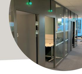
The kuando Busylight IoT for LoRaWAN® networks is a Class C LoRaWAN® device and can be installed in large variety of use cases. Through the LoRaWAN® downlink package the kuando Busylight can be programmed to show any color and used as a visual notifier, indicating a certain event, status or as a cue for specific handling. Installing the Busylight in networks combined with Class A sensors will complete the IoT experience and the use cases are basically endless.
