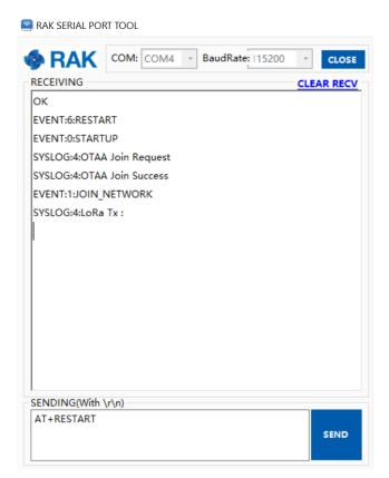
Figure 11: RAK7431 Successful Join
