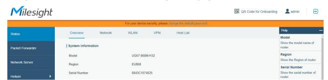
C. Fill in the wallet address in hotspot web GUI and click "Generate" to generate the QR code.
