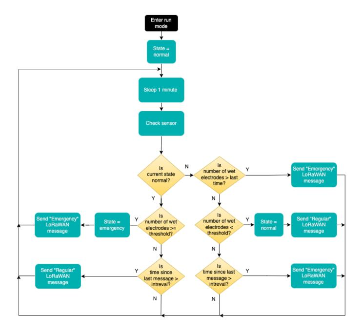
When the device enters its run mode, its state is set to normal, and it checks for the presence of water on each electrode every minute (check <u>Sensor Dimension and Electrode Definition</u> to see what an electrode is). By default, 4 electrodes need to be wet for the device to sense a leak.
