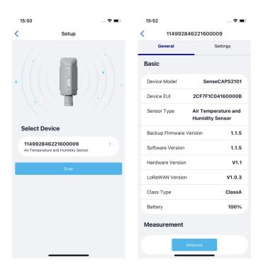
4) Enter configuration mode after Bluetooth connection is successful: LED flashes at 2s frequency.
