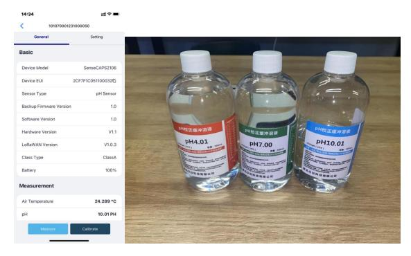
2) Prepare the standard liquid and pour an appropriate amount of the liquid into the graduated cylinder. Insert the pH probe electrode into the liquid in the
