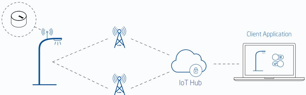
Luminaire controlling solution enables remote lighting control for LED luminaires with DALI. With better control over lighting you are able to reduce energy consumption, CO2 emission as well as allow efficient maintenance cycles.
