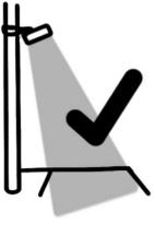
When mounted on a pole or mast you should point the sensor to the middle of the road (center line). This can be done easily by adjusting the tiltable bracket MT80-15. The bracket can be placed about 3-4 meters above ground. Please check the max range of the sensor. **Important: The pole must not move in the wind**
