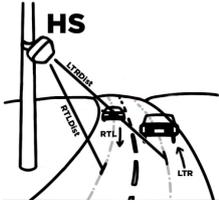
**Two lanes, cross traffic (2L2D)** This is typical for HS applications such as measuring traffic on interstate roads. RTLDist and LTRDist are different.
