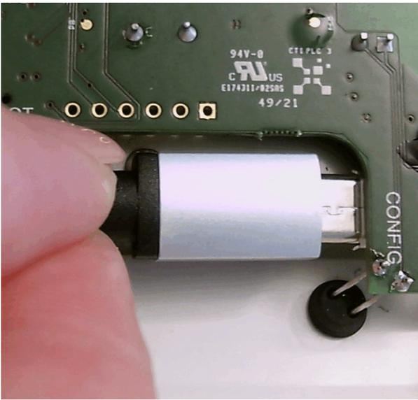
Note: On first generation TCR units (TCR-LS, TCR-LSS, TCR-HS, TCR-HSS), the configuration port is located on the main board. To connect the USB cable, the unit must be opened.
