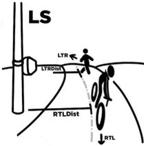
**Cross traffic on one lane (1L2D)** This is typical for low speed traffic (LS) measuring bicycle lanes or small paths. In this case get the distance to the center of the track and set RTLDist and LTR Dist to the same value.
